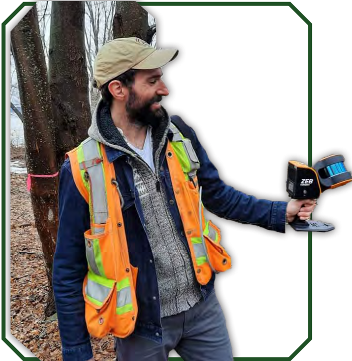
Above: GeoSLAM unit for on the ground data collection.
